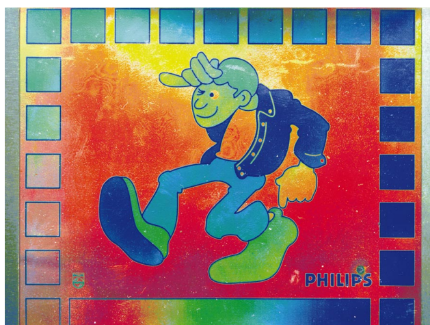
Fig. 10 Photograph of a sample patternwise exposed to UV light.
